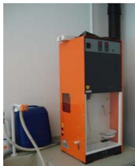
Distillation apparatus for ammonium
