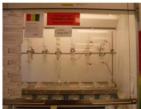
Soxhlet apparatus for lipids
