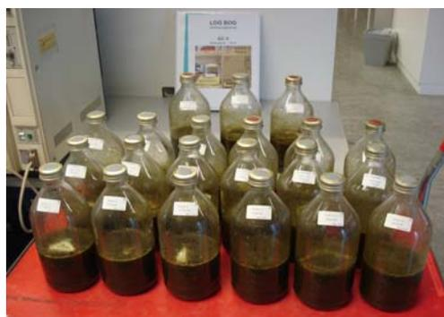
**Figure 3** Batch experiment of biogas potential using glass bottles
